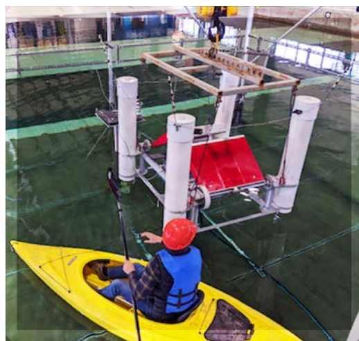
At Oregon State University's Hinsdale Wave Research Lab, a researcher works with a wave energy converter device in the wave basin. TEAMER is opening the doors to our nation's best marine energy testing facilities and the experts who work there. Photo by Hinsdale Wave Research Lab
