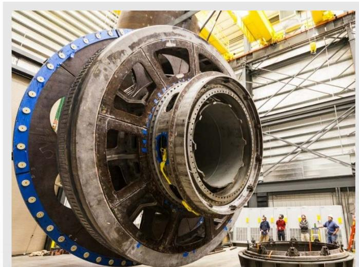
Figure 33. Columbia Power Technologies' wave energy converter is installed at NREL's 5-MW dynamometer at its Flatirons Campus.
