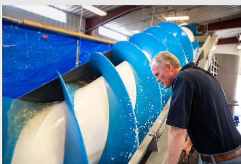
Figure 17. Percheron Power's composite Archimedes hydrodynamic screw.
