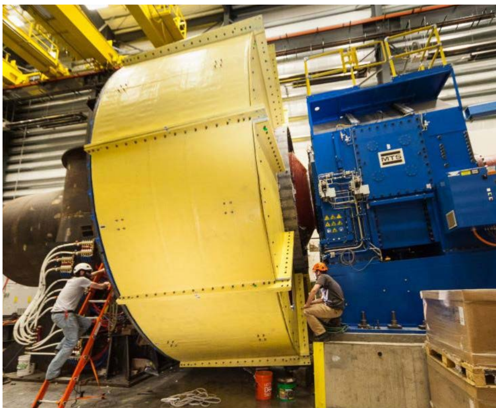
C-Power's wave energy system undergoing testing at NREL's Flatirons Campus
