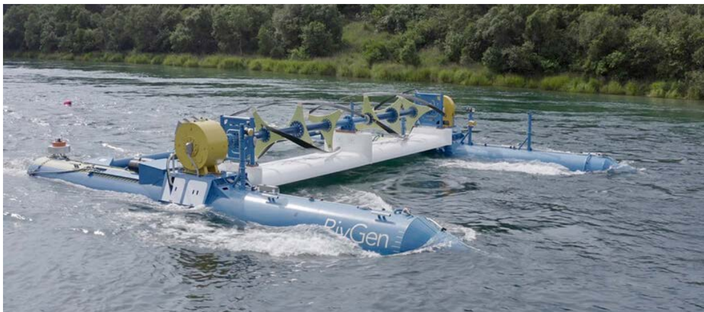
RivGen® by ORPC during deployment in the Kvichak River near Igiugig, Alaska
