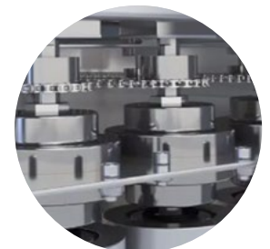
Patented external magnetic couplers drive the internal robotics
