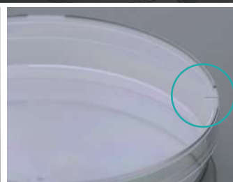
Vent points for Gas Exchange
