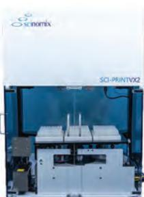
The Sci-print VX2 is a fully automated tube and vial labeler capable of handling a broad range of tube sizes. In addition to print and apply automation, the Sci-print VX2 can be configured to sort racked tubes, receive bulk tubes, uncap/recap, fill and/or scan barcodes.
