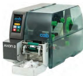
The Axon 2 is a low throughput volume tube and vial label applicator offering reduced operator involvement when compared to manual labeling. The operator places the tube or vial in the applicator arms, taps the touchscreen icon and the labeled tube is either dropped into the tray or removed by hand.
