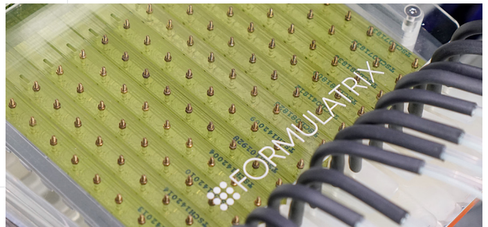
Each 8-nozzled microfluidic chip dispenses reagents rapidly with minimal waste.
