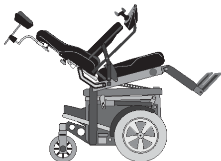
Figure 2. Front-wheel drive power wheelchair with recline capability.
