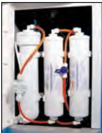
Filter assembly is front door accessible
